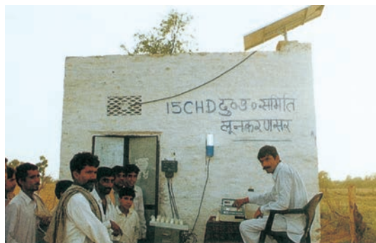
Fig. 5.10: Solar operated electronic milk testing equipment
