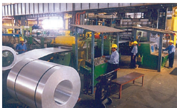
Fig. 6.3: Strip casting mill at smelter of NALCO
